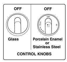
To Replace: Hold the knob with the OFF position up, so that the control knob stem opening on the underside of the knob aligns with stem. Push knob down. Do not force the knob onto the stem.
